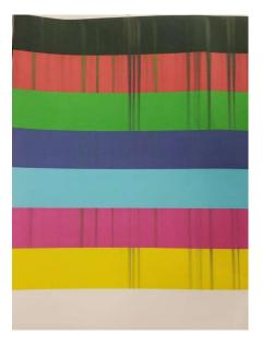
**NOTE**: The "Print Color Bars" test print pattern, shown here, can be performed using the "Print Color Bars" button, located in the "Test Print Menu" on the Printer's Touchscreen.
