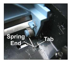
7. Gently insert a small, flathead screwdriver between the blue Printhead Latch Pin and the black plastic hinge [A] and rotate to pop the Printhead Latch out of the hinge without damaging either piece.
