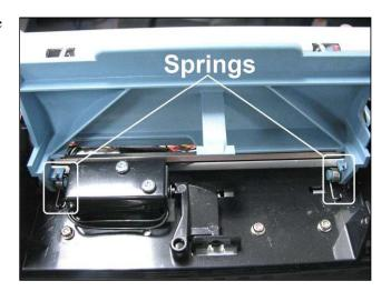
6. Use needle-nose pliers or tweezers to gently pull the rounded end of the Spring out from beneath the plastic tab in the housing and remove the Spring. Repeat the procedure to remove the second Spring.
