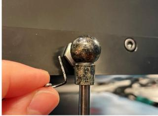
**7.** Holding the printhead from below to provide support, remove the gas lift. Drop the printhead head down slowly with the gas lift disconnected.
