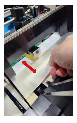
2.3. If necessary, some feeders have three positions for the separator foot, you may move it to any of the three positions that best centers the foot on the envelope size you are running. You can move the separation foot to the proper position to achieve this.
