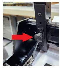
Lift the pin and give it a quarter turn to hold the pin in the up position, slide the guide to the proper location, turn the pin back and move the guide back and fourth slightly so that the pin pops into the groove and hole. This will lock the guide into place.
