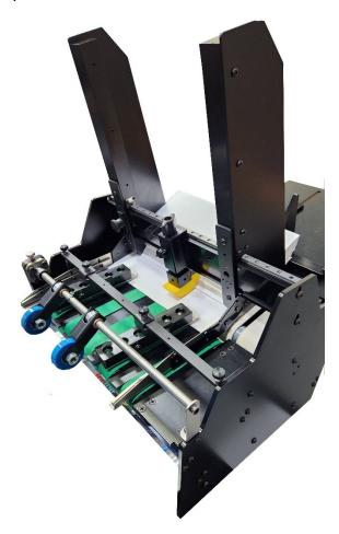
This feeder has an alignment section (green belts) that will drive the envelope against the non-operator side edge guide. This will help to straighten the envelope before it is fed onto the blue belt. Setting the feeder up properly is important to get consistent and straight feeding. Follow this step by step guide to get the best feeding.
