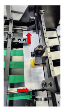
3.2. Tighten the locking screw to make sure the guide does not move while printing.
