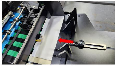
4.2. Note that the position of the wedge can affect how well the sheets are separated and fed. At times you may be required to move the wedge forward or back a bit to achieve the best feeding.
