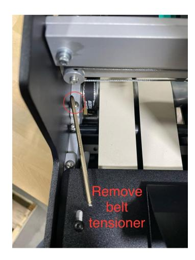
9. Remove the screws which tension the motor and secure the motor plate.
