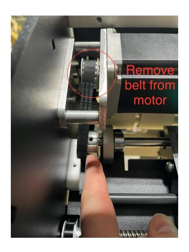
12. Remove the four screws securing the feed motor to the motor plate.
