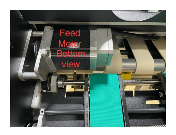
7. To access the motor, remove the bottom plate of the feeder.
