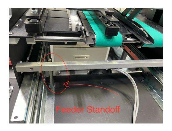
5. With the feeder pulled out, remove the six screws located below the feeder. There are three screws per side. Have a second person ensure the feeder does not tip or it will cause serious damage. Lift the feeder straight up.
