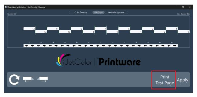
The highlighted button will send a job to the printer. This job has color bars for each color on each die to easily identify any necessary changes.
