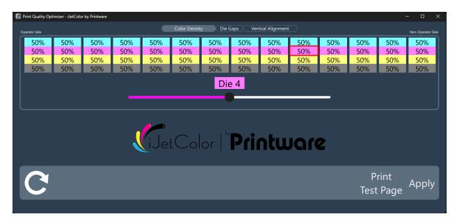
In the above image, magenta on die 4 has been selected for adjustment. There is a red rectangle around the color that has been selected. Moving the slider to the right will make the color more dense or darker (100%), and moving it to the left will make it less dense or lighter (0%). When a color is selected for adjustment, it will be highlighted with a red rectangle. The color of the slider will change to match the selected color.
