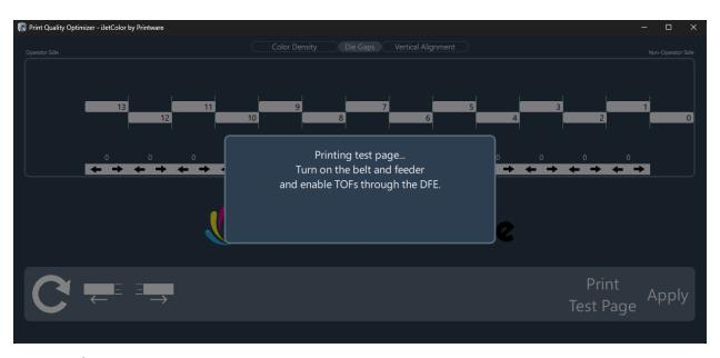
After the job has been sent to the printhead, this popup appears, instructing the operator to turn on the belt and feeder and enable TOFs. These operations are not done automatically.
