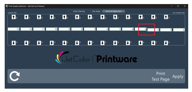
In the image above, die 3 has been moved up as far as it can be moved. Notice the offset value is 6 for die 3, but even though all the dies to the left of die 3 have also moved, their values are still 0 because the offset value is relative to the die to its right.
