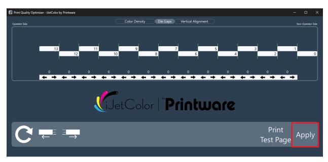
The highlighted button will display a list of all the changes to be applied to the printhead. The changes will include all the visible values for die gaps, vertical alignment, and color density.
