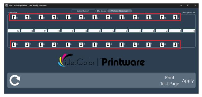
The buttons to move each individual die are highlighted in the red rectangles above. Die 0 is assumed to be perfectly aligned from the factory, so all dies are adjusted relative to it. Notice the small digits to the right of each button. These digits are a visual representation of the current alignment setting.
