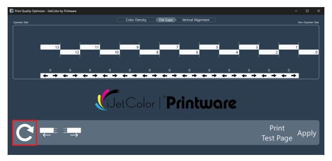
The highlighted reset button will reset die gap and vertical alignment values to 0 and color density values to 50% for all colors and all dies.
