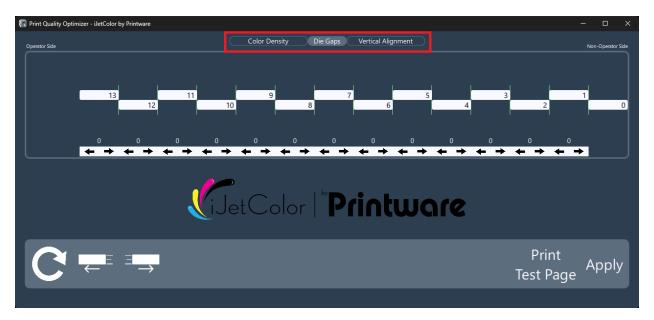
To navigate to the color density and vertical alignment menus, select one of the highlighted tabs.
