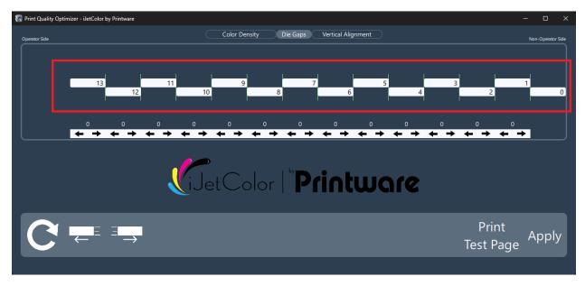
The dies are physically arranged in a zigzag pattern on the printhead, so they are represented in the same zigzag pattern onscreen inside the red rectangle. The dies are numbered 0 to 13 with die 0 being the furthest on the non-operator side and 13 furthest on the operator side.
