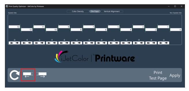
This button moves all dies, except die 0, to the left, thus creating gaps between all the dies. You will notice from the animation that die 13 moves closer to the operator side of the printer. This is what physically happens on the printhead. The resulting print may appear slightly wider than if all the dies were moved to the right.
