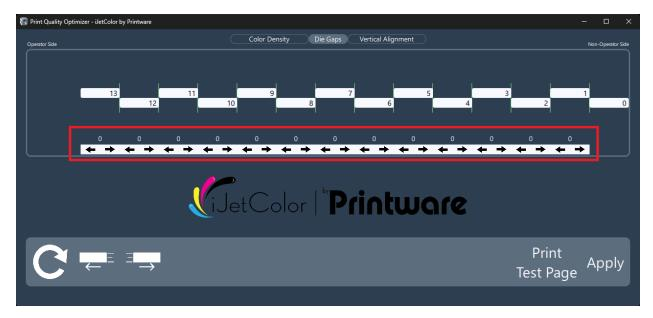
Each die in the die gaps menu, except die 0, can be moved to the left or right. This movement occurs with respect to the die immediately to the right of it. For example, moving die 4 to the left will increase the gap between dies 3 and 4, while the gaps between all other dies remain the same. If you move one die several notches one direction, you will notice all the dies to the left of it move the same distance in the same direction.
