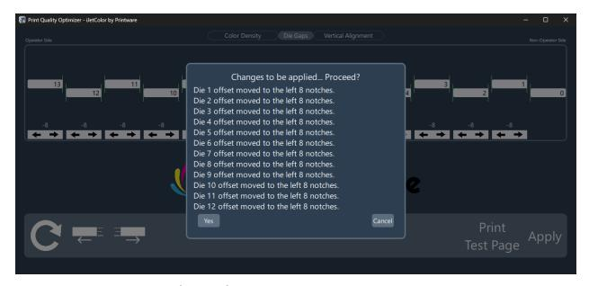
This is an example of a list of changes to be made. This list is scrollable. In this case, all the dies have been moved to the left.
