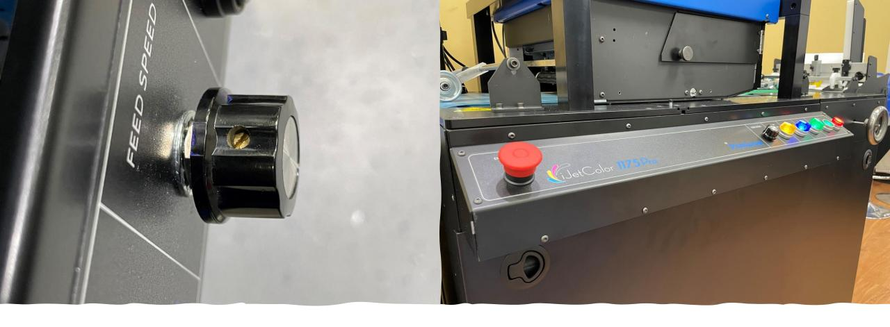
Replace the speed adjustment pot for Pro+ Feeder – Front Panel and Feed Speed
