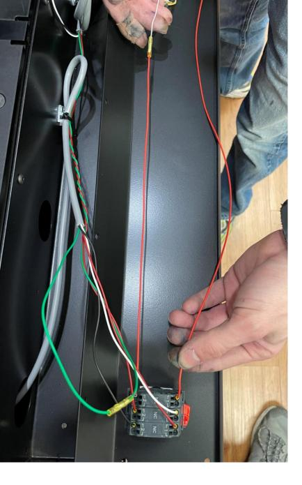
Replace the speed adjustment pot for Pro+ Feeder – Install New Pot  When installing the new speed adjustment pot the pot has white wires. Note that red wires are soldered on as extensions and the wiring is the same as the old speed adjustment pot.
