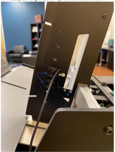
7. Place the Auto-Loader Feeder atop the shelf and connect the new feeder guide to the Auto-Loader Feeder.
