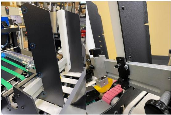
5. Swap the current feeder backplate with the new feeder backplate. The backplate is secured with four  $3/32^{nd}$  inch screws.
