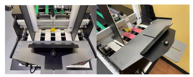
6. The new non-operator side guide has a sensor that is height adjustable. The Auto-Loader will feed until envelopes reach the set sensor level. Set the height of the sensor to change how many envelopes are always stored in the feeder.
