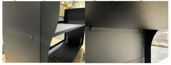
7. Mount the tabletop on the cart top and secure with screws. Each screw goes through on the top holes and washers followed by a nut secure from below.
