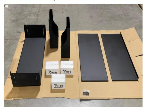
4. Mount the sides to the bottom of the cart using the screws provided. The screw goes on the outside. The washer followed by the nut secure the screw from the inside. *Mount the side panel so there are four open holes above the top screw as pictured below.*
