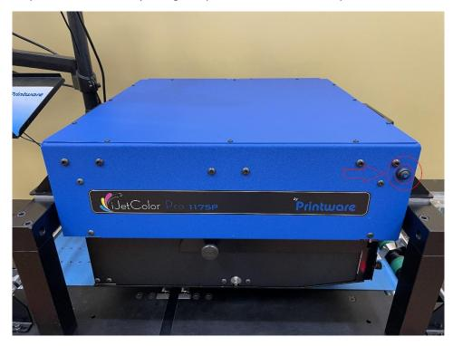
**4.** Once the front power light turns off, switch off the printhead power rocker switch on the back of the printhead.
