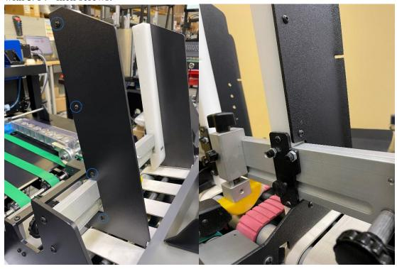
4. Swap the current feeder backplate with the new feeder backplate. The backplate is secured with four 3/32<sup>nd</sup> inch screws.
