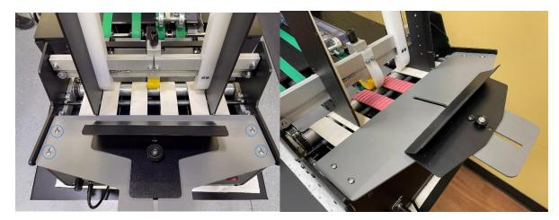
5. The new non-operator side guide has a sensor that is height adjustable. The Auto-Loader will feed until envelopes reach the set sensor level. Set the height of the sensor to change how many envelopes are always stored in the feeder.
