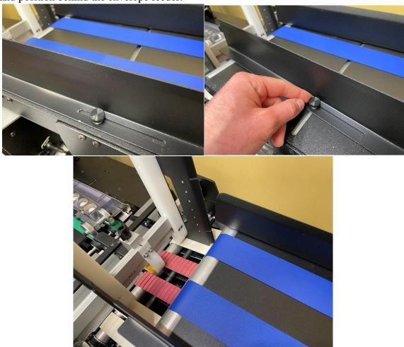
8. Connect the power and turn on the Auto-Loader. The speed can be adjusted using the knob and the sensor can be ignored by selecting "Continuous Run".
