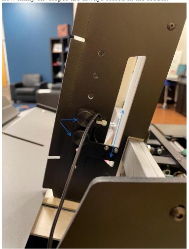
6. Place the Auto-Loader Feeder atop the shelf and connect the new feeder guide to the Auto-Loader Feeder.
