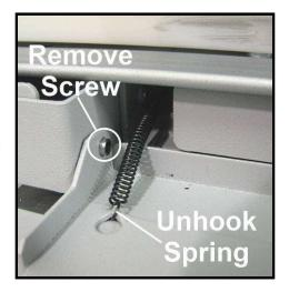
**7. Remove Top Cover.** Remove "cover pivot screw", at non-operator side. Remove Top Cover and set aside.
