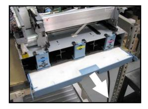
2. Remove Engine Base. Remove (6) T-10 screws, (3) on each side) of the Print Engine Assembly. (Set aside for reassembly).
