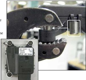
bar for example) to provide even pressure to press the insert in partially. Then use pliers or another tool to press the insert the rest of the way in.
