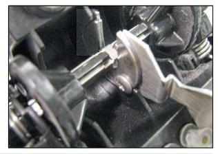
**NOTE:** The Wrench fits around the shaft as shown. Please be sure that the Wrench head and the screw head [**D**] fit around the Pinch Valve housing Rib; as shown.
