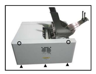
**5. Remove Front Exit Cover** by removing (4) screws.
