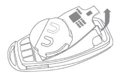
3 Replace the battery and reinstall the cover
