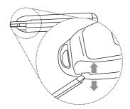
2 Remove the mainboard from the housing
