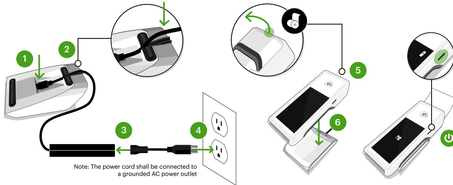
Note: The power cord shall be connected to a grounded AC power outlet
